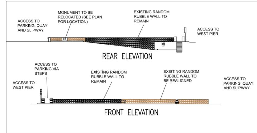
ACCOMMODATION ROAD – WALL REALIGNMENT – EXISTING WALL ELEVATION
