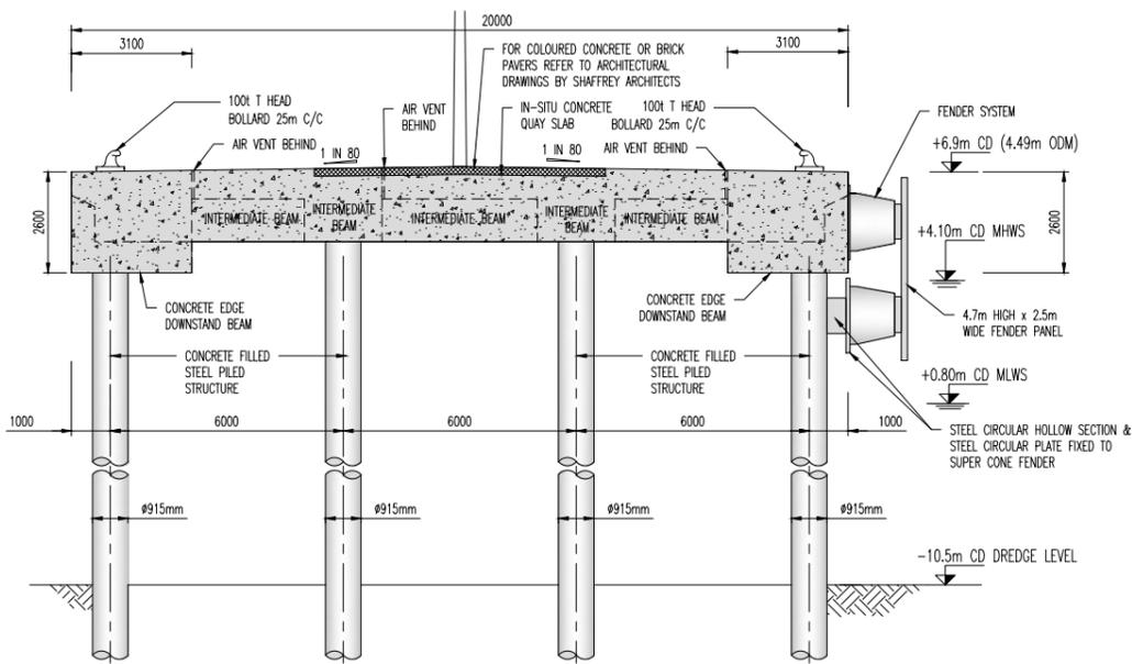
CROSS SECTION OF FIXED QUAY STRUCTURE AT FENDER PILE
