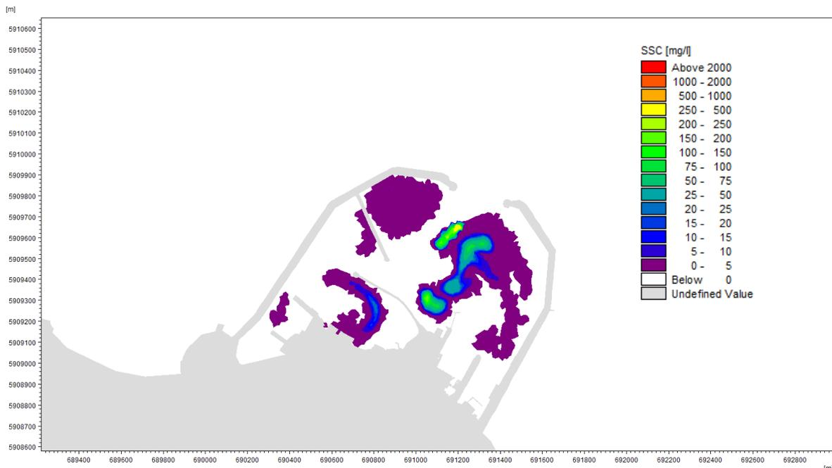
Figure 19. Increase in SSC Resulting from Continuous Dredging of Silty Sediment in Dun Laoghaire Harbour (Spring Tide, High Water Slack)
