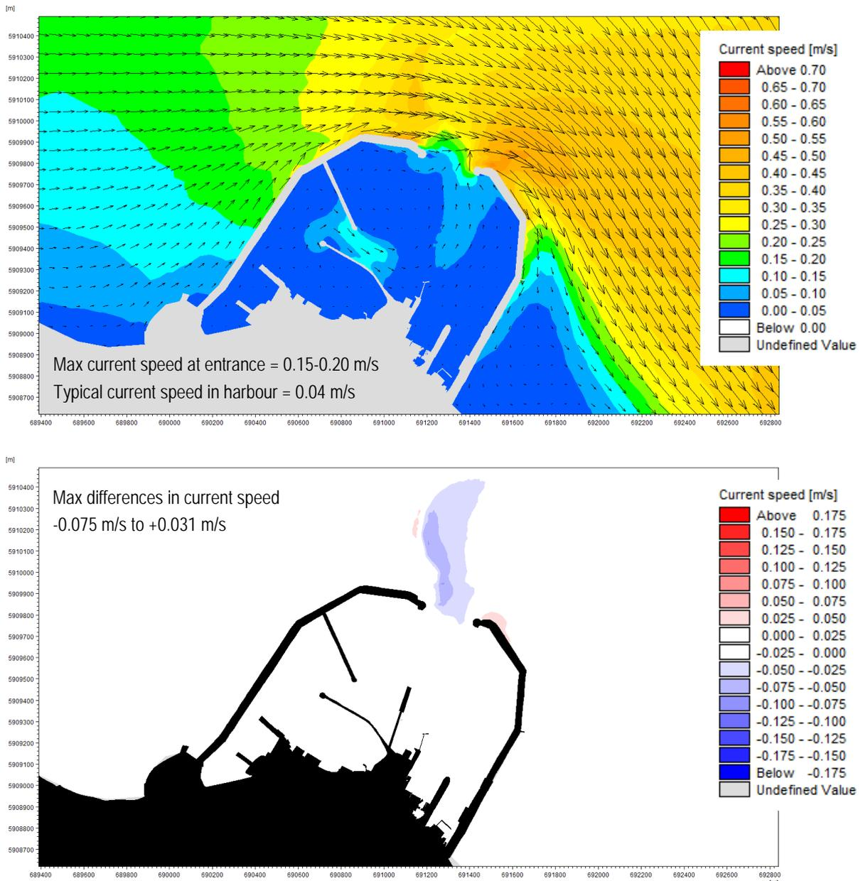
Figure 43. Baseline Tidal Current Speed (Top) and Difference in Current Speed (Bottom) as a Result of the Scheme (Mean Spring Tide, HW+3hrs, Peak Ebb).
