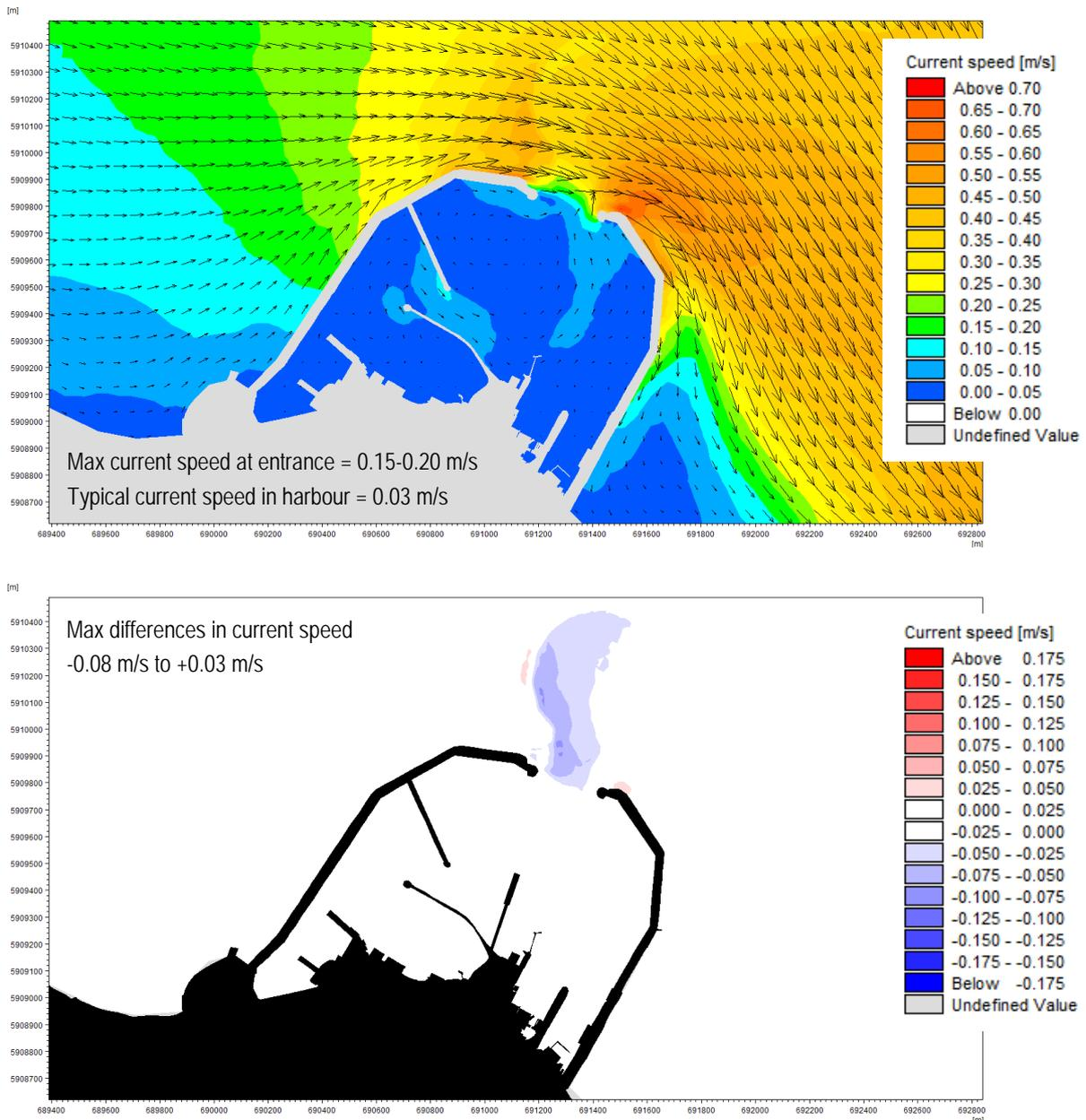
Figure 42. Baseline Tidal Current Speed (Top) and Difference in Current Speed (Bottom) as a Result of the Scheme (Mean Spring Tide, HW+2hrs, Ebb)
