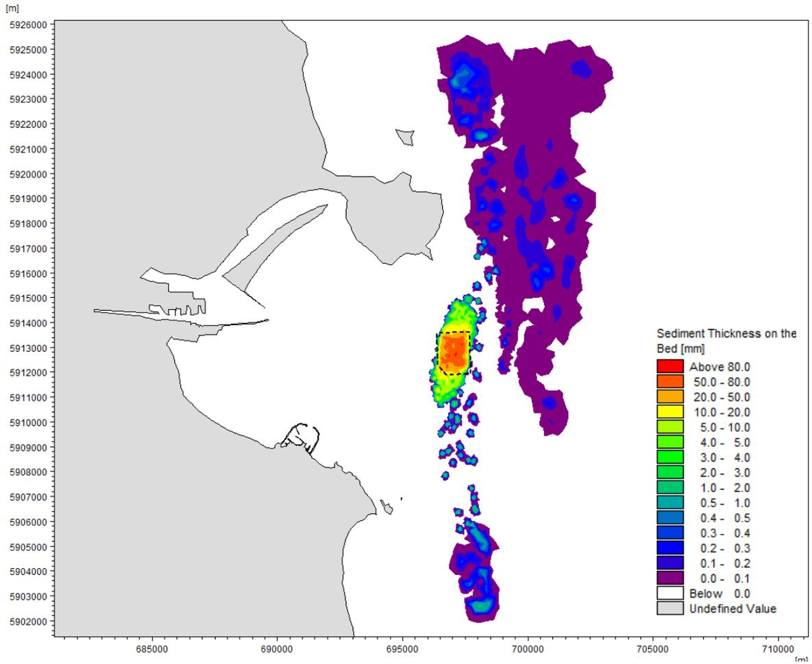
Figure 35. Sediment Deposition Thickness Resulting from Deposition of All Sandy and Silty Sediment at the Burford Bank Spoil Ground
