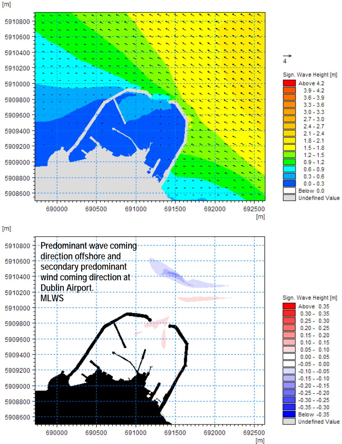
Figure 53. Baseline Significant Wave Height (Top) and Difference in Significant Wave Height (Bottom) as a Result of the Scheme (Scenario S10 [1:50, 170/120, MLWS])
