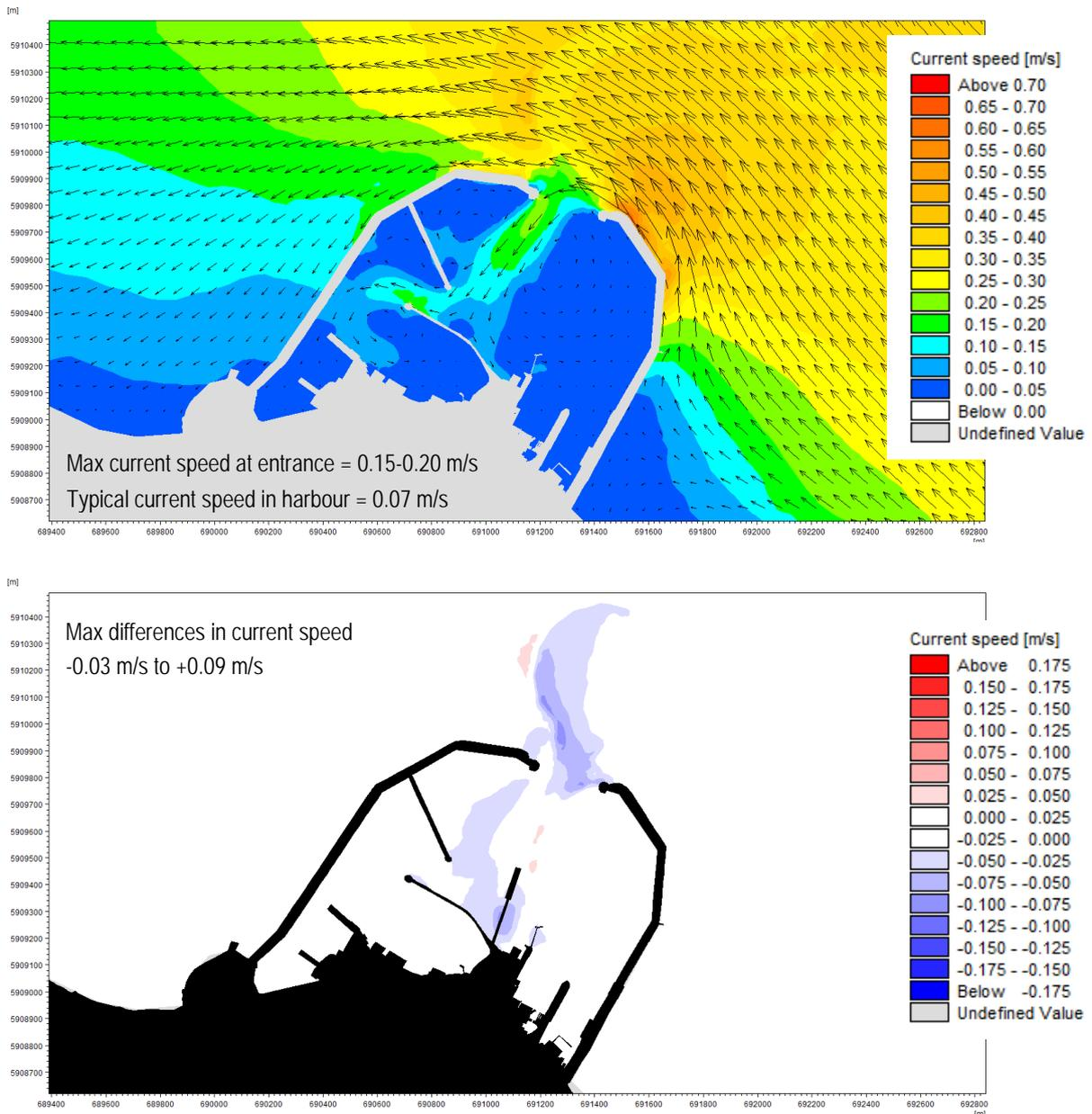
Figure 37. Baseline Tidal Current Speed (Top) and Difference in Current Speed (Bottom) as a Result of the Scheme (Mean Spring Tide, HW-3hr, Peak Flood).
