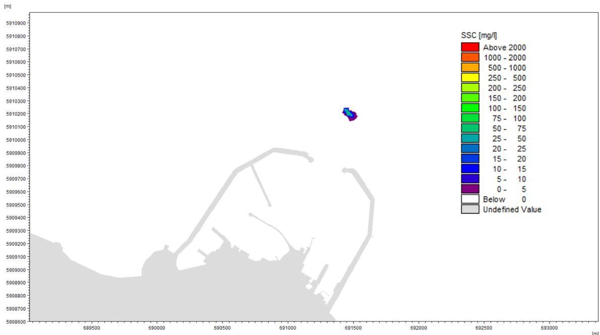
Figure 28. Increase in SSC Resulting from Continuous Dredging of Sandy Sediment outside Dun Laoghaire Harbour (Spring Tide, Peak Ebb Currents)
