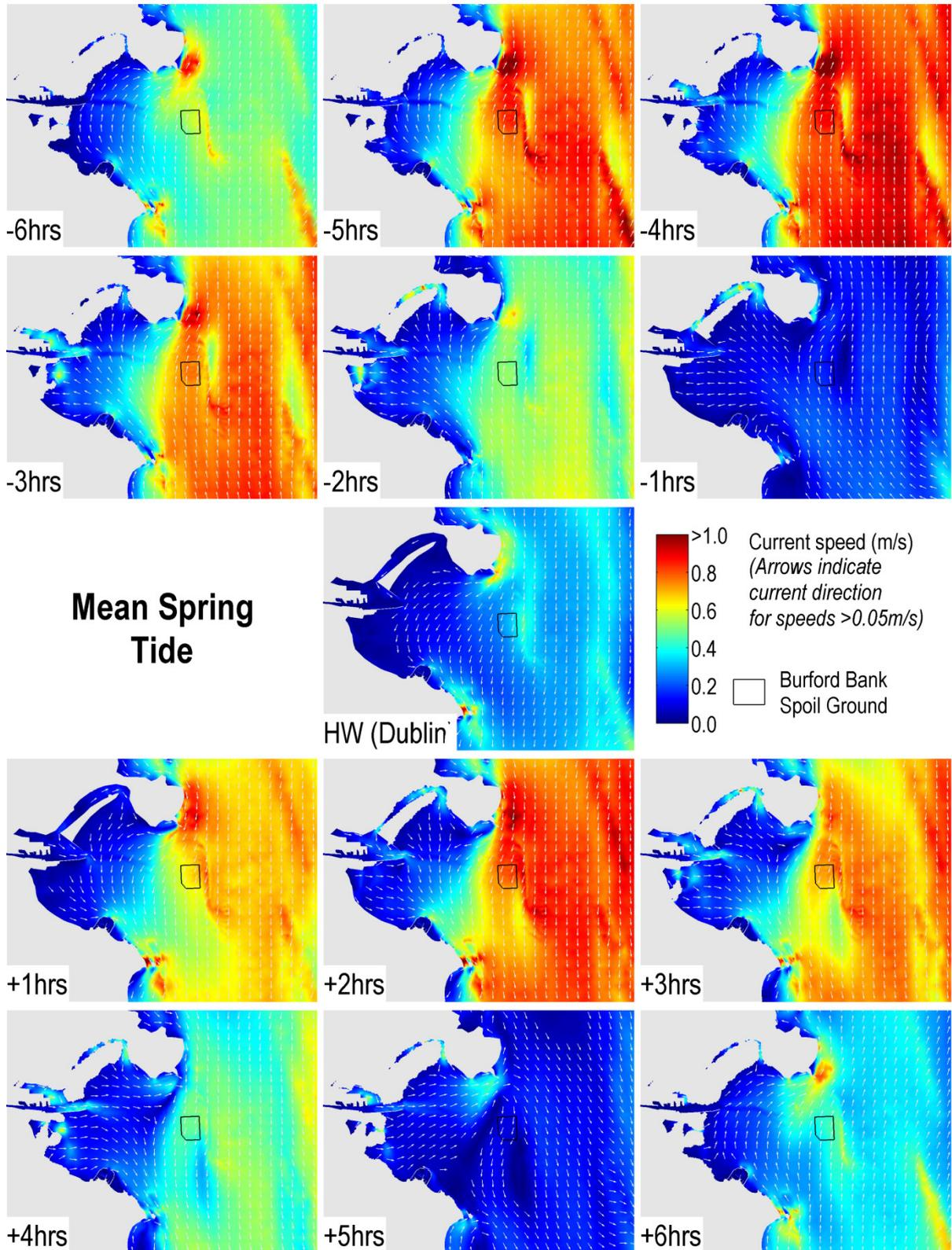
Figure 13. Mean Spring Tidal Currents in the Region of Dublin Bay
