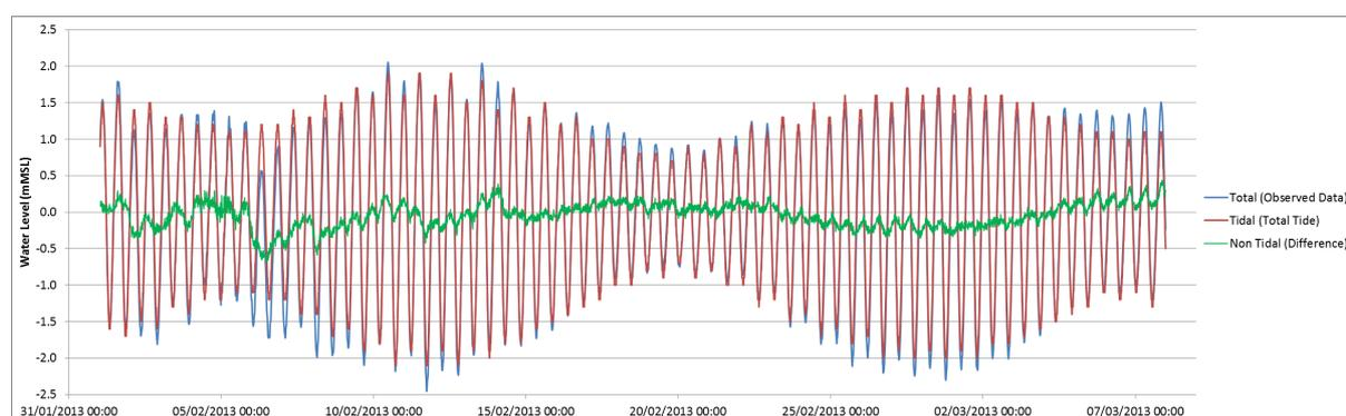
Figure 60. Comparison of Total, Tidal and Non-tidal Water Levels at Dublin Port
