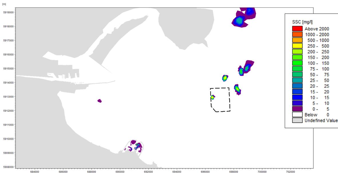
Figure 31. Increase in SSC Resulting from Continuous Dredging of Silty Sediment inside Dun Laoghaire Harbour and Subsequent Disposal at Burford Bank Spoil Ground (Spring Tide, High Water Slack)
