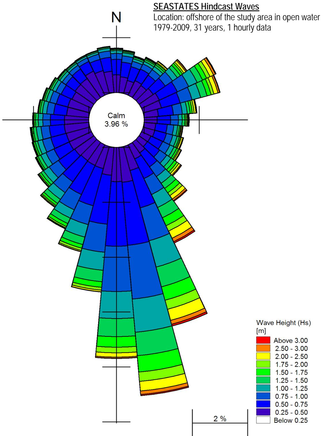
Figure 10. Offshore Wave Climate
