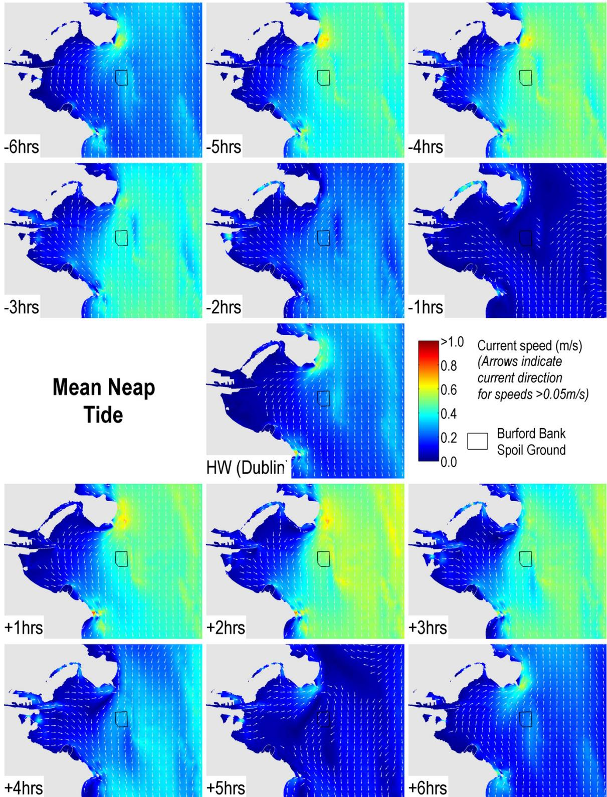
Figure 14. Mean Neap Tidal Currents in the Region of Dublin Bay
