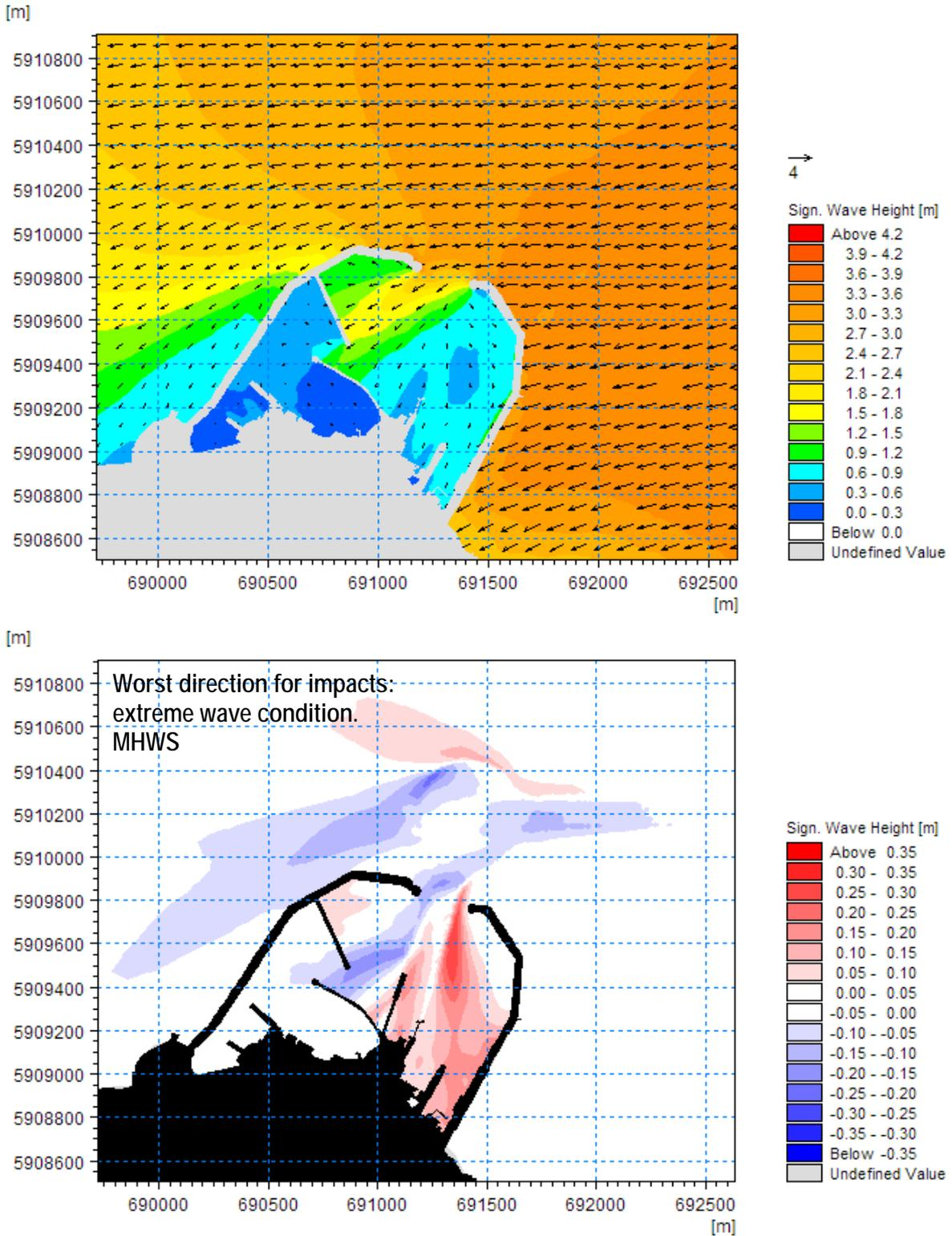
Figure 48. Baseline Significant Wave Height (Top) and Difference in Significant Wave Height (Bottom) as a Result of the Scheme (Scenario S5 [1:50, 60/85, MHWS])
