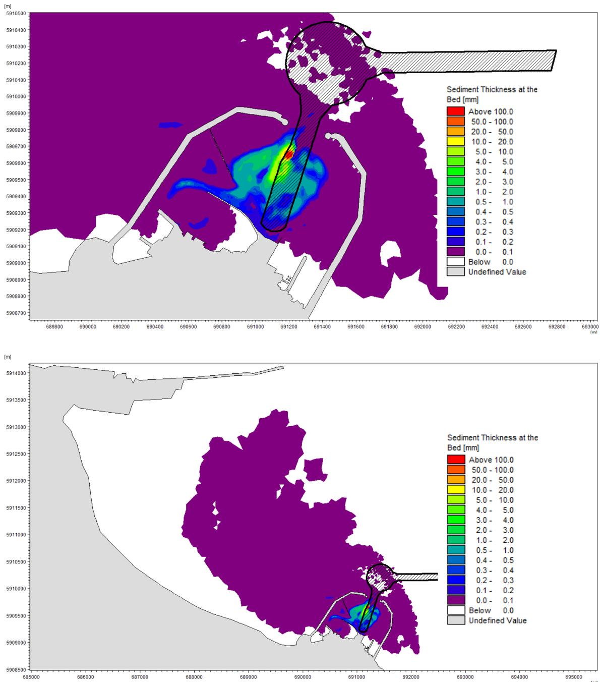
N.B. The black hatched area indicates the footprint of the dredged channel
