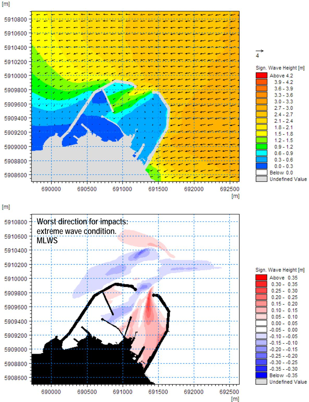
Figure 49. Baseline Significant Wave Height (Top) and Difference in Significant Wave Height (Bottom) as a Result of the Scheme (Scenario S6 [1:50, 60/85, MLWS])
