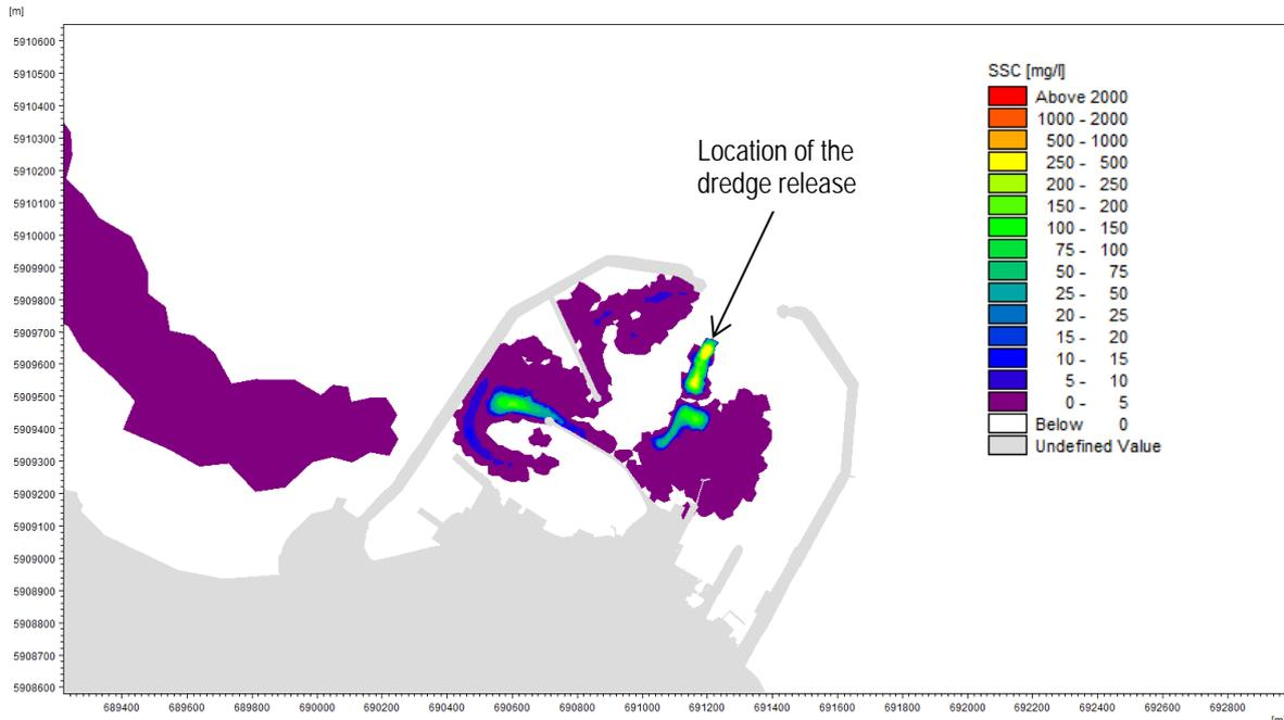
Figure 18. Increase in SSC Resulting from Continuous Dredging of Silty Sediment in Dun Laoghaire Harbour (Spring Tide, Peak Flood Currents)
