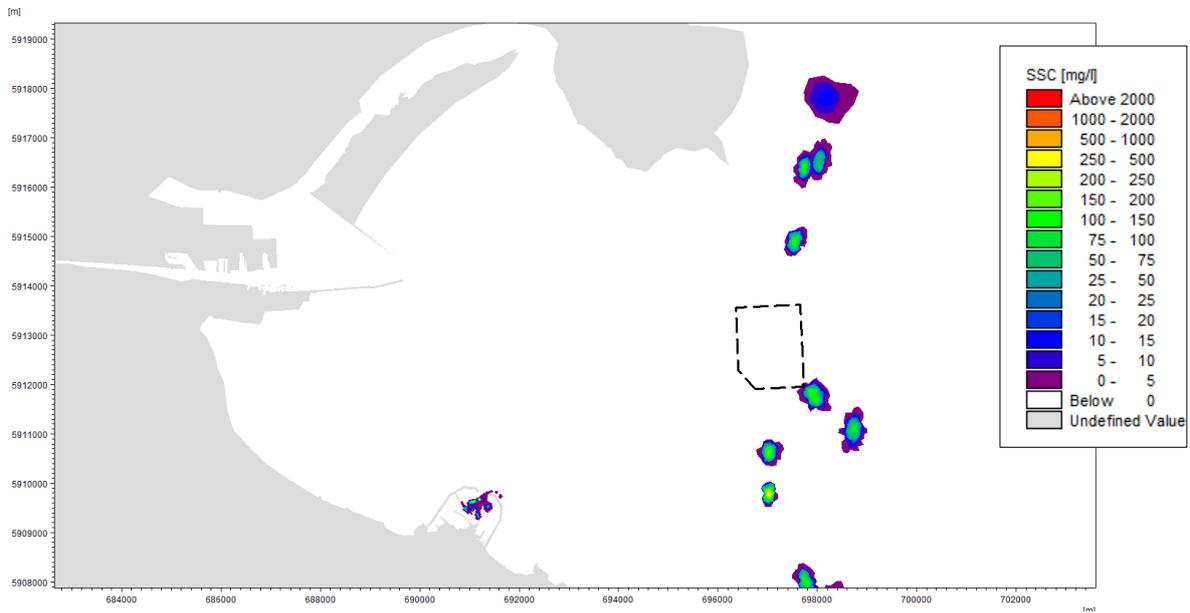
Figure 32. Increase in SSC Resulting from Continuous Dredging of Silty Sediment inside Dun Laoghaire Harbour and Subsequent Disposal at Burford Bank Spoil Ground (Spring Tide, Peak Ebb Currents)
