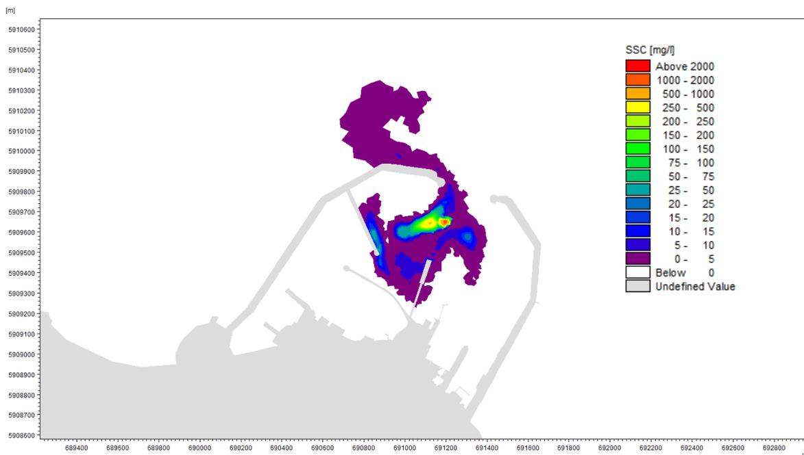
Figure 25. Increase in SSC Resulting from Continuous Dredging of Silty Sediment in Dun Laoghaire Harbour (Neap Tide, Low Water Slack)
