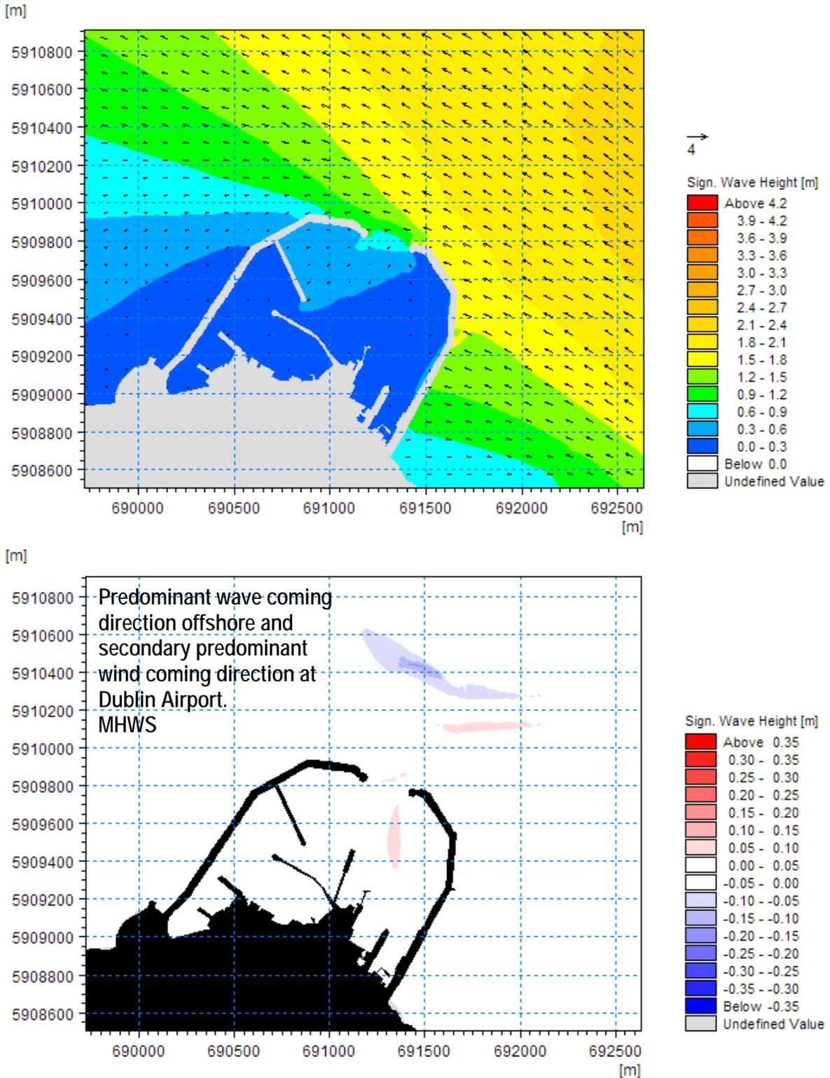
Figure 52. Baseline Significant Wave Height (Top) and Difference in Significant Wave Height (Bottom) as a Result of the Scheme (Scenario S9 [1:50, 170/120, MHWS])
