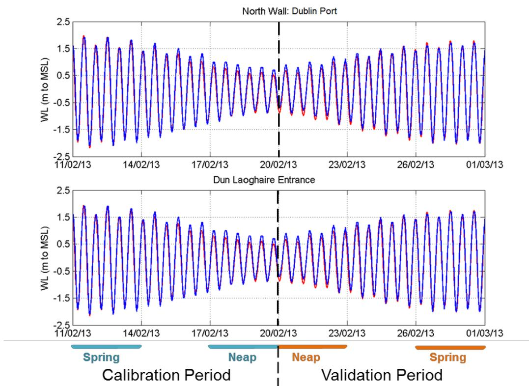
Figure 61. Comparison of Modelled Tidal Water Levels (Blue) with TT Predicted Tidal Water Levels for Dublin Port (Red)
