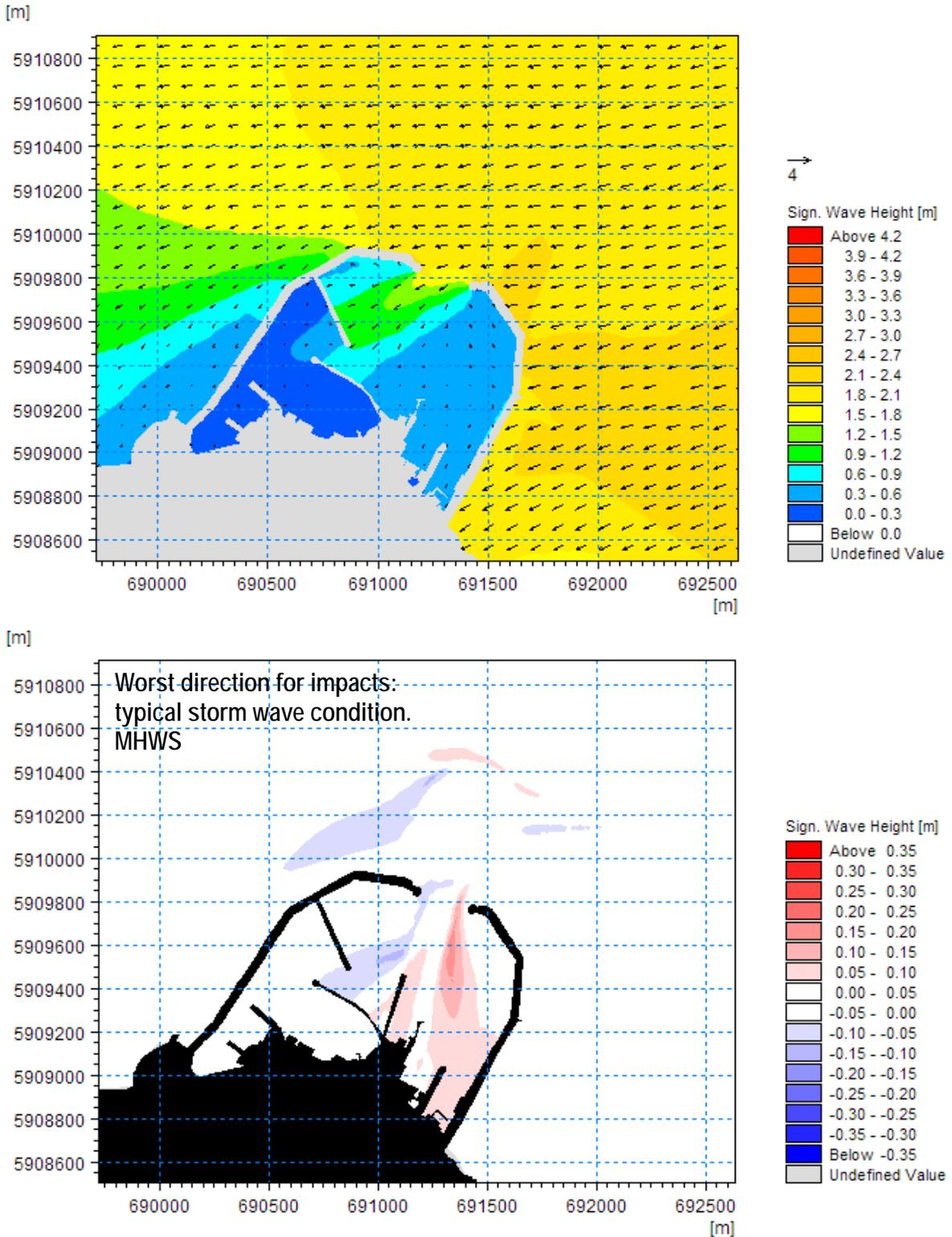
Figure 44. Baseline Significant Wave Height (Top) and Difference in Significant Wave Height (Bottom) as a Result of the Scheme (Scenario S1 [10:1, 60/85, MHWS])
