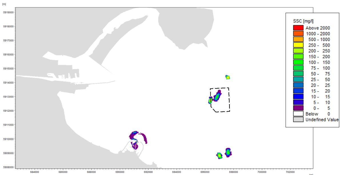
Figure 33. Increase in SSC Resulting from Continuous Dredging of Silty Sediment inside Dun Laoghaire Harbour and Subsequent Disposal at Burford Bank Spoil Ground (Spring Tide, Low Water Slack)
