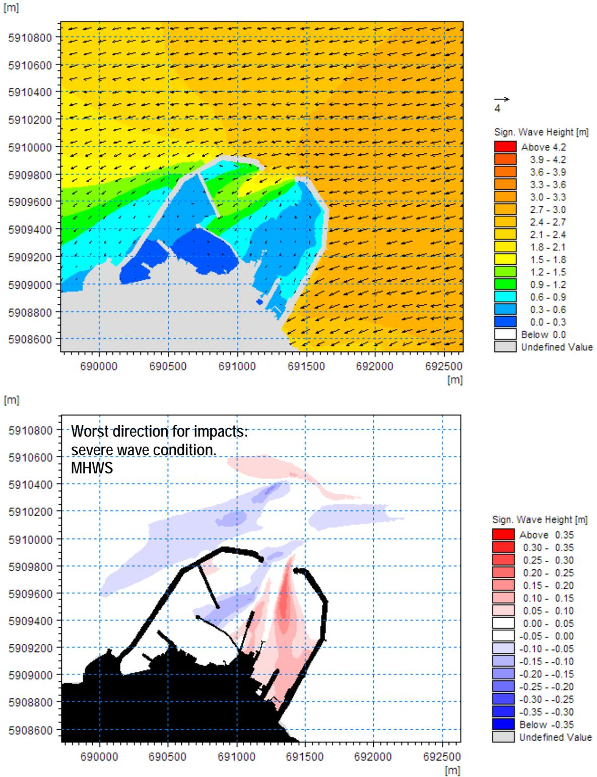
Figure 46. Baseline Significant Wave Height (Top) and Difference in Significant Wave Height (Bottom) as a Result of the Scheme (Scenario S3 [1:1, 60/85, MHWS])
