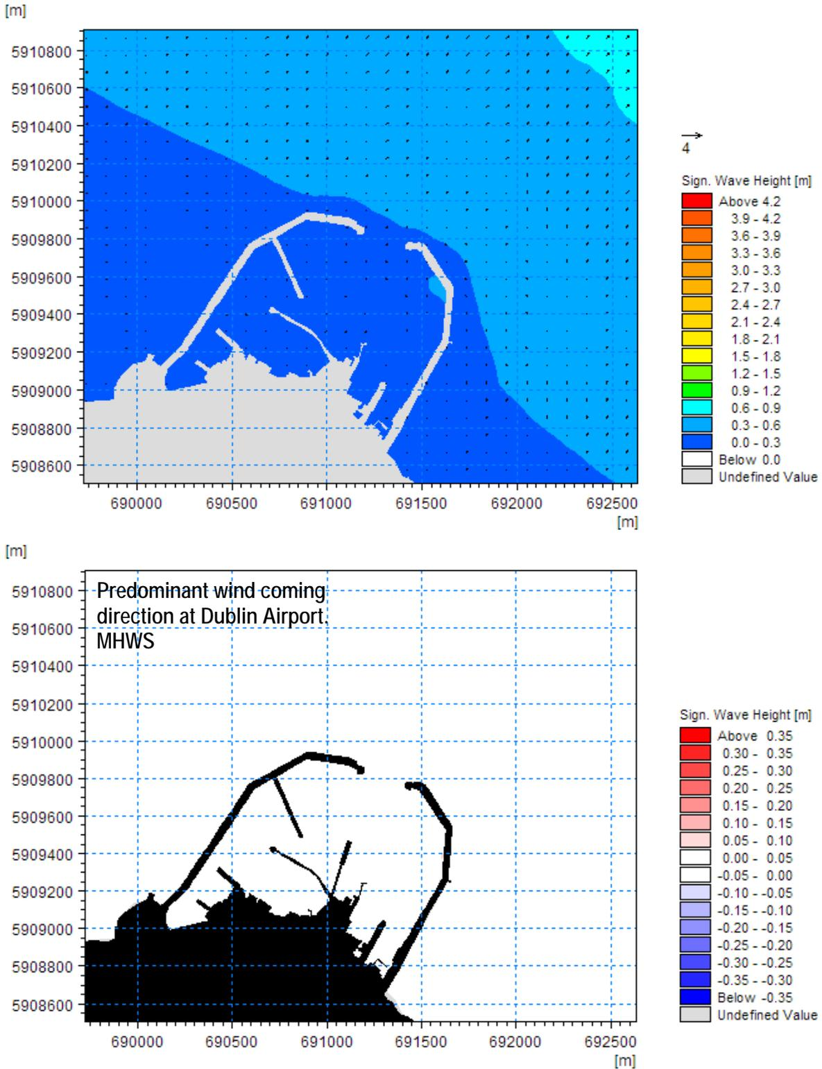
Figure 50. Baseline Significant Wave Height (Top) and Difference in Significant Wave Height (Bottom) as a Result of the Scheme (Scenario S7 [1:50, 240/230, MHWS])
