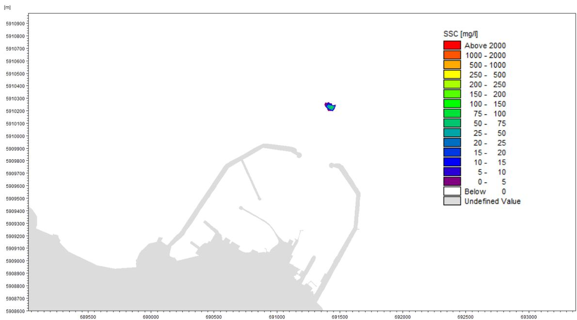
Figure 29. Increase in SSC Resulting from Continuous Dredging of Sandy Sediment outside Dun Laoghaire Harbour (Spring Tide, Low Water Slack)
