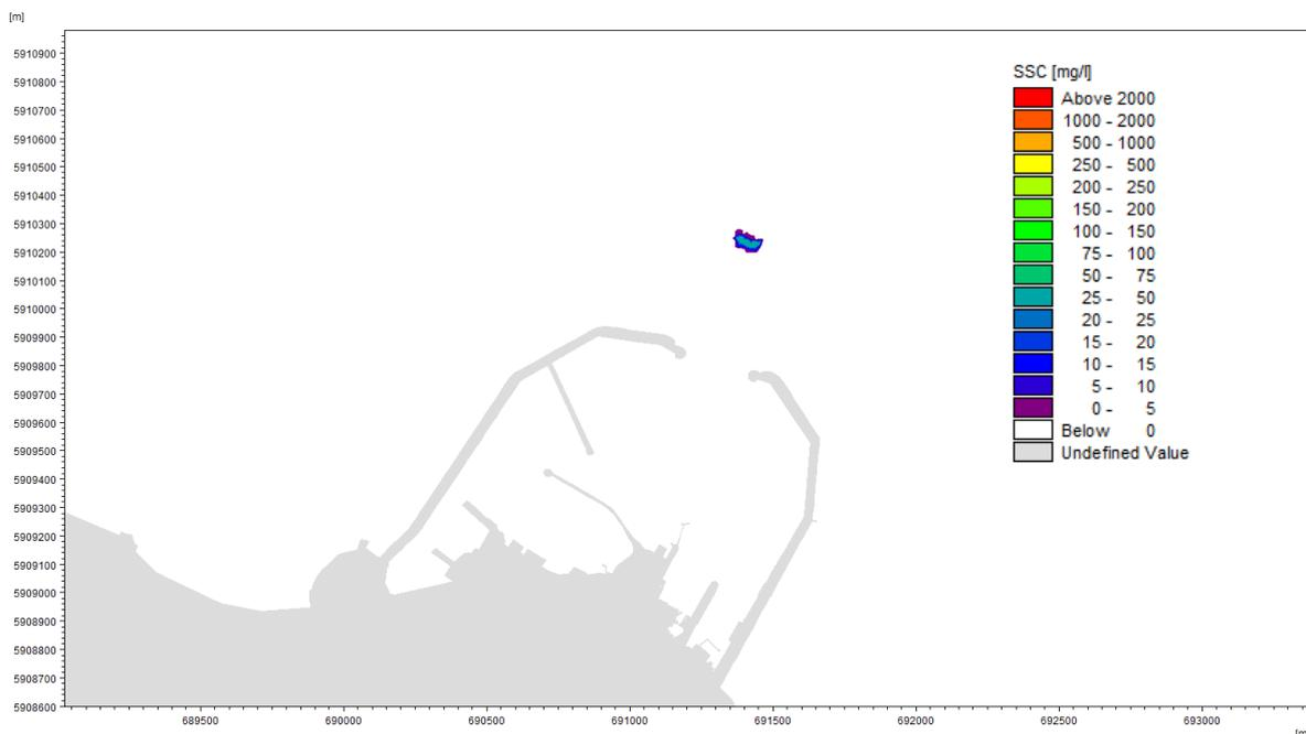
Figure 26. Increase in SSC Resulting from Continuous Dredging of Sandy Sediment outside Dun Laoghaire Harbour (Spring Tide, Peak Flood Currents)
