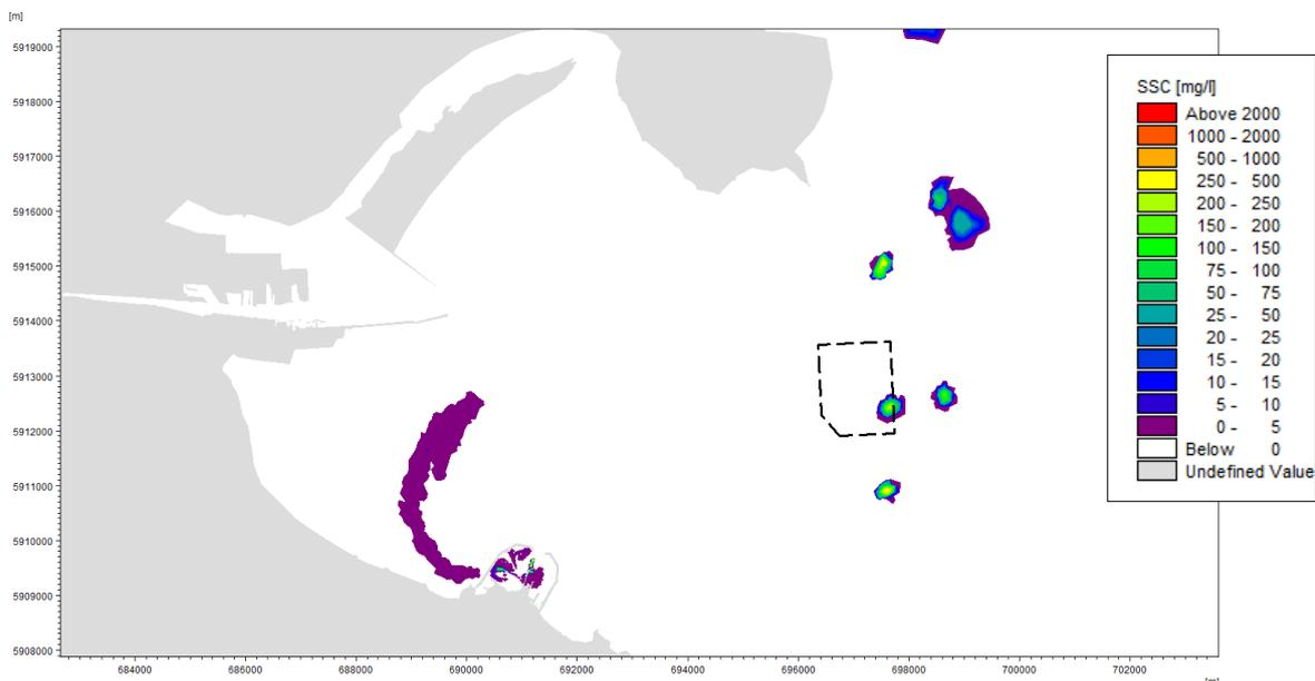
Figure 30. Increase in SSC Resulting from Continuous Dredging of Silty Sediment inside Dun Laoghaire Harbour and Subsequent Disposal at Burford Bank Spoil Ground (Spring Tide, Peak Flood Currents)
