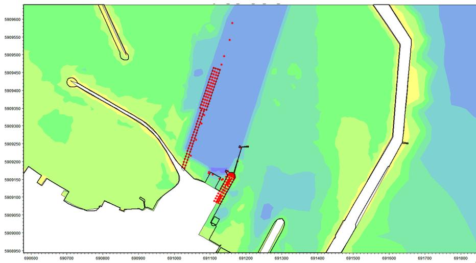
Figure 58. Locations of Existing and New Scheme Piles Simulated in the Tide and Wave Models
