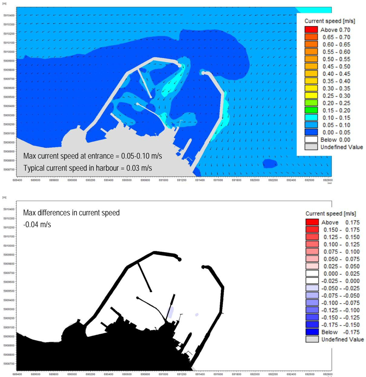
Figure 39. Baseline Tidal Current Speed (Top) and Difference in Current Speed (Bottom) as a Result of the Scheme (Mean Spring Tide, HW-1hrs, Flood)
