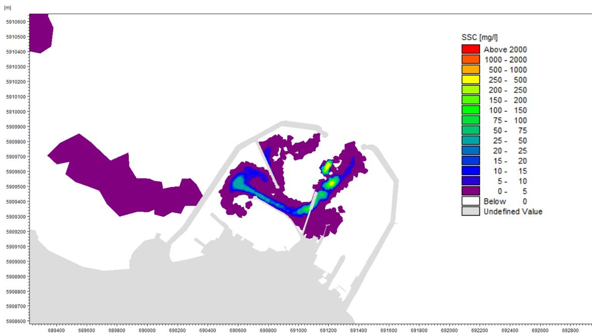
Figure 22. Increase in SSC Resulting from Continuous Dredging of Silty Sediment in Dun Laoghaire Harbour (Neap Tide, Peak Flood Currents)
