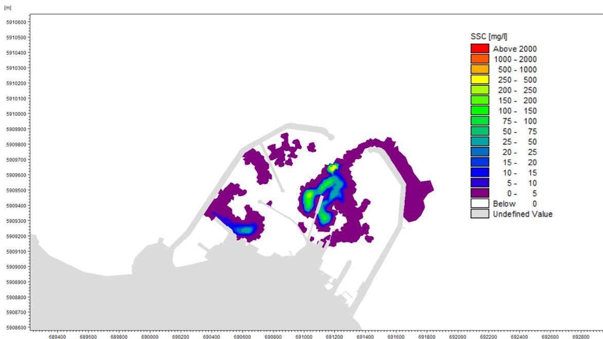
Figure 23. Increase in SSC Resulting from Continuous Dredging of Silty Sediment in Dun Laoghaire Harbour (Neap Tide, High Water Slack)
