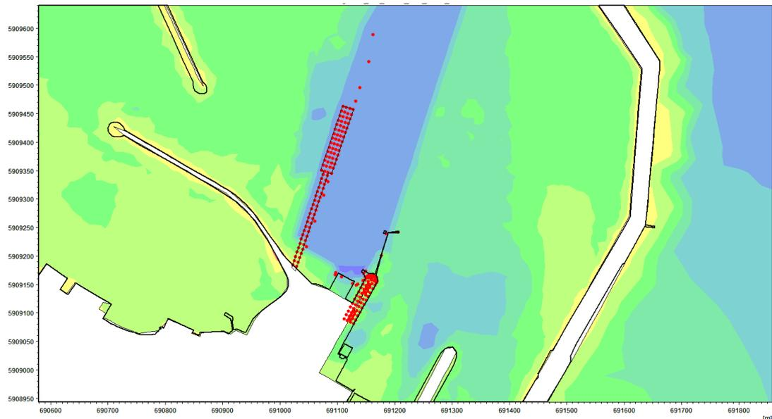
Figure 36. Locations of Existing and New Scheme Piles Simulated in the Tide and Wave Models
