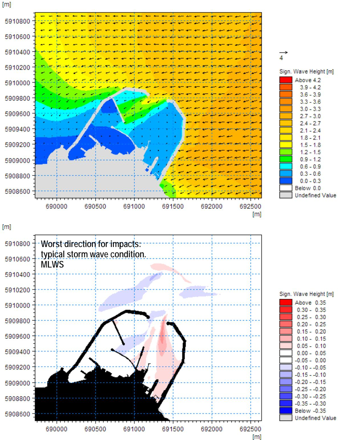
Figure 45. Baseline Significant Wave Height (Top) and Difference in Significant Wave Height (Bottom) as a Result of the Scheme (Scenario S2 [10:1, 60/85, MLWS])
