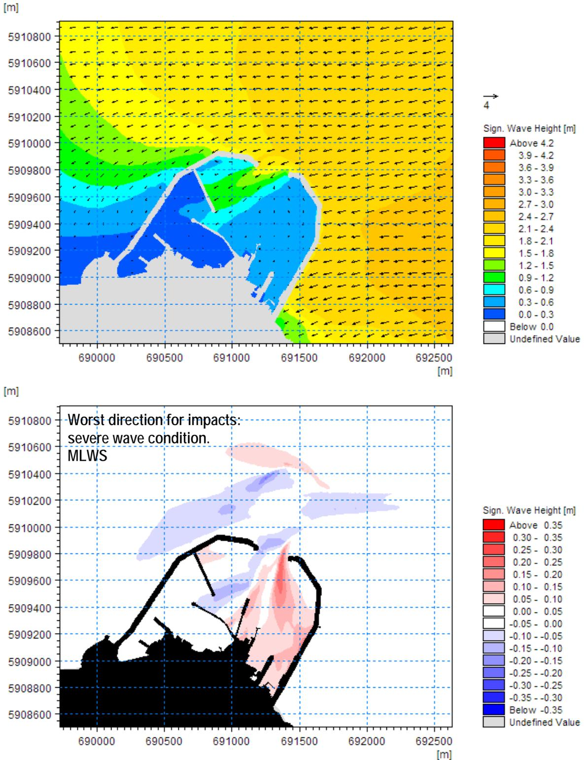
Figure 47. Baseline Significant Wave Height (Top) and Difference in Significant Wave Height (Bottom) as a Result of the Scheme (Scenario S4 [1:1, 60/85, MLWS])
