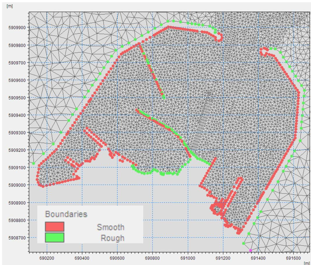
Figure 62. Distribution of Reflective Boundary Types in the Wave Model
