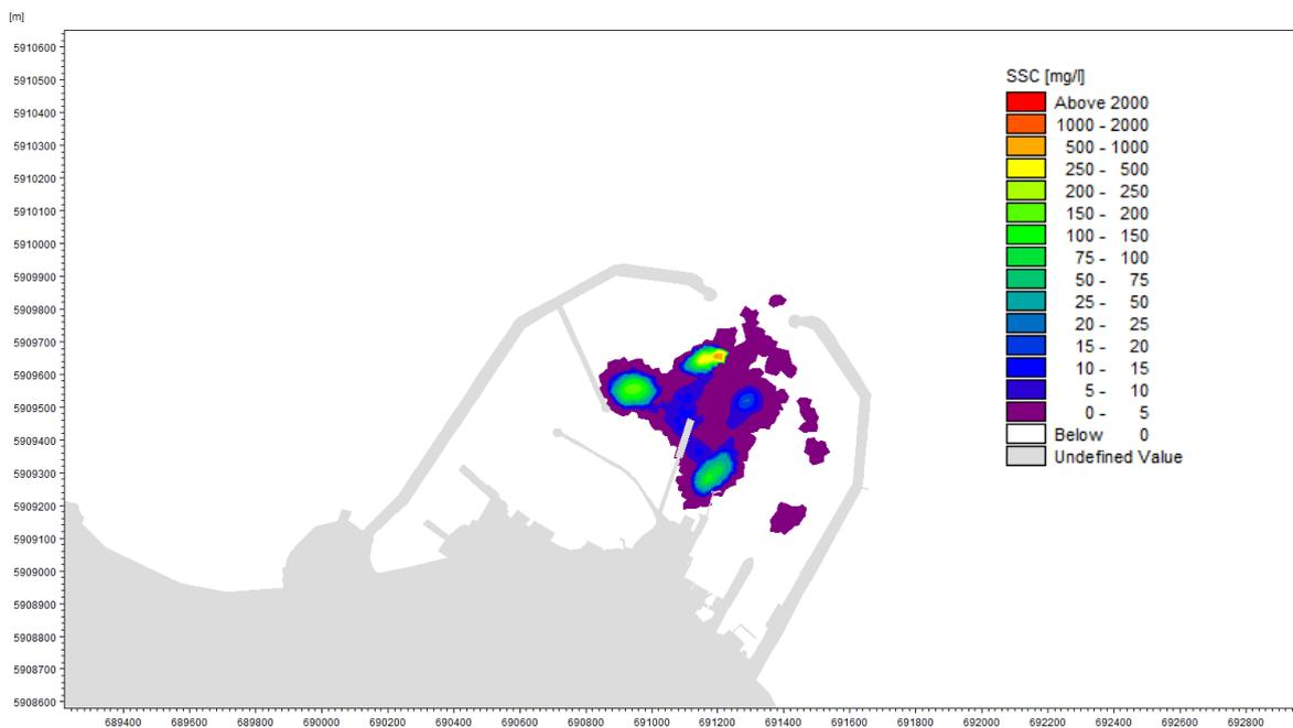
Figure 24. Increase in SSC Resulting from Continuous Dredging of Silty Sediment in Dun Laoghaire Harbour (Neap Tide, Peak Ebb Currents)
