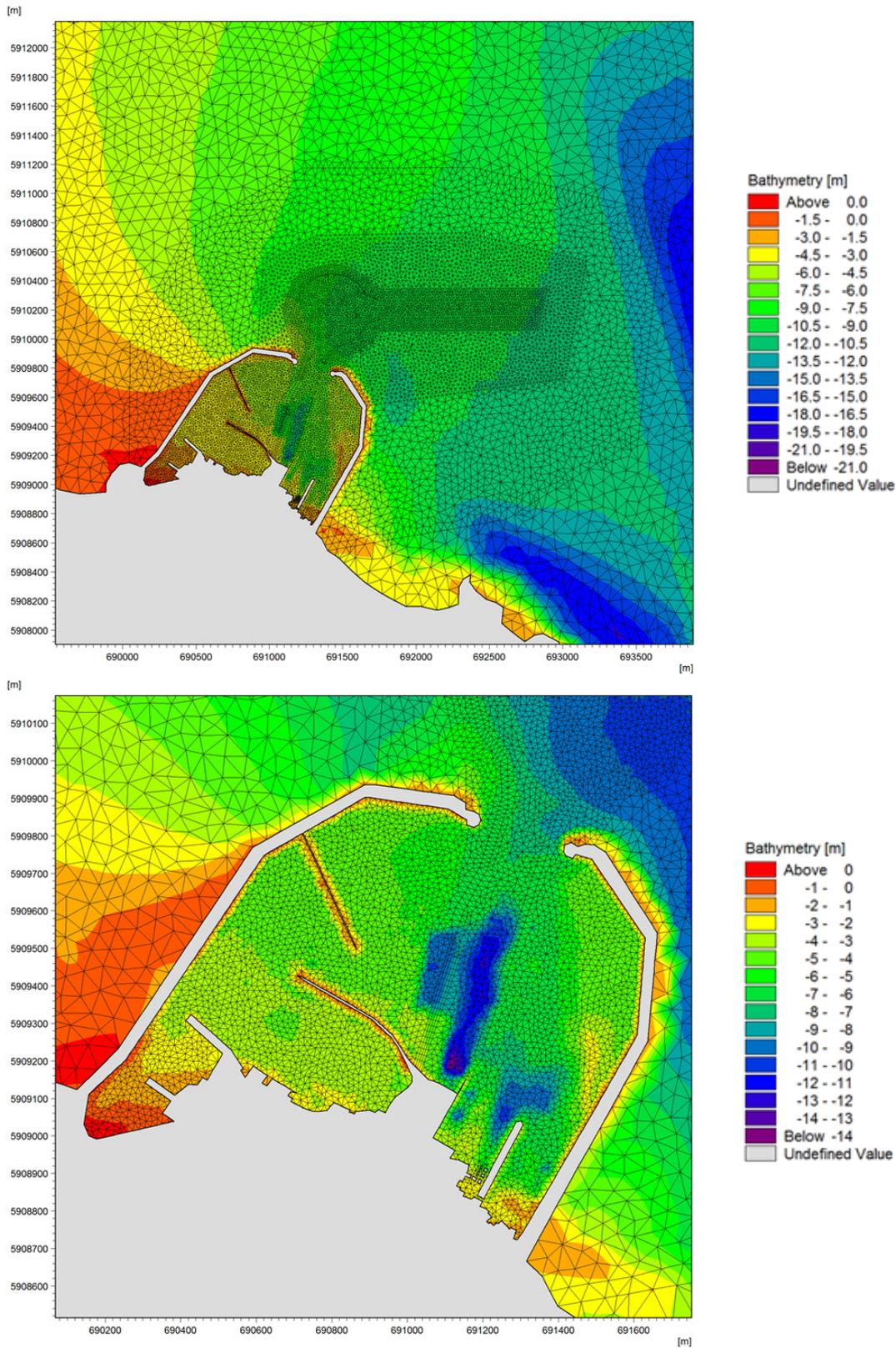
Figure 56. Detail of the Model Mesh Within Dun Laoghaire Harbour
