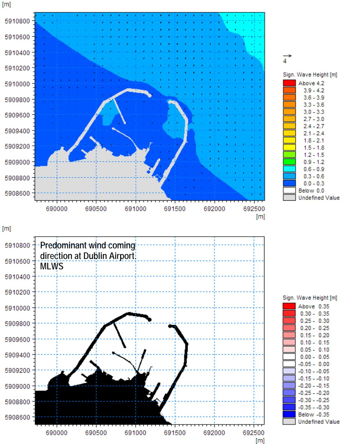
Figure 51. Baseline Significant Wave Height (Top) and Difference in Significant Wave Height (Bottom) as a Result of the Scheme (Scenario S8 [1:50, 240/230, MLWS])
