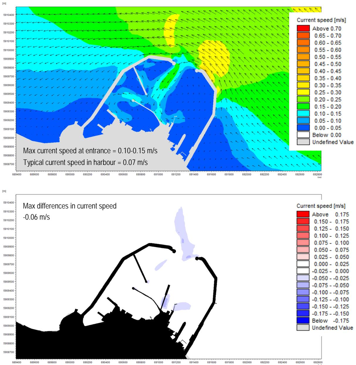
Figure 38. Baseline Tidal Current Speed (Top) and Difference in Current Speed (Bottom) as a Result of the Scheme (Mean Spring Tide, HW-2hr, Flood)
