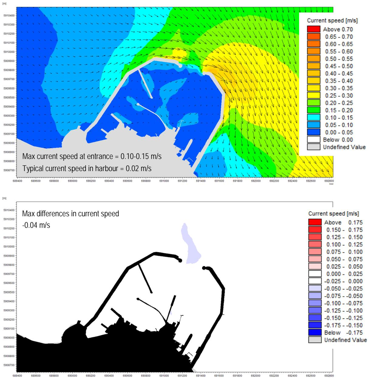
Figure 40. Baseline Tidal Current Speed (Top) and Difference in Current Speed (Bottom) as a Result of the Scheme (Mean Spring Tide, HW Slack)
