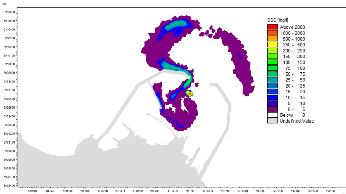
Figure 21. Increase in SSC Resulting from Continuous Dredging of Silty Sediment in Dun Laoghaire Harbour (Spring Tide, Low Water Slack)
