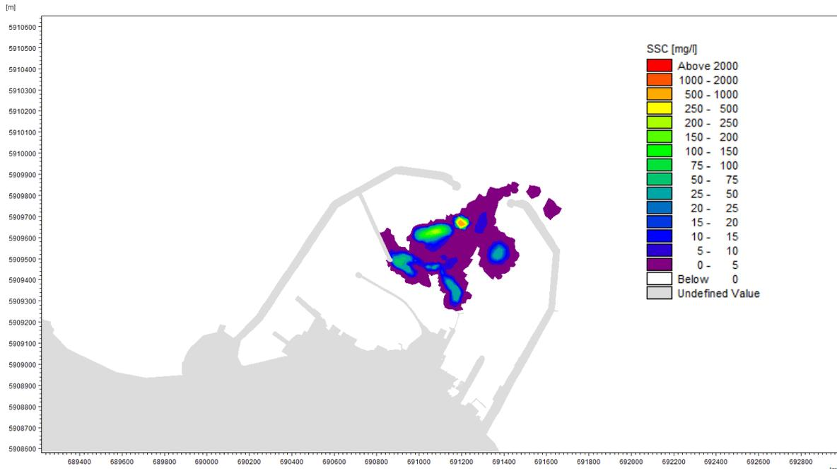
Figure 20. Increase in SSC Resulting from Continuous Dredging of Silty Sediment in Dun Laoghaire Harbour (Spring Tide, Peak Ebb Currents)
