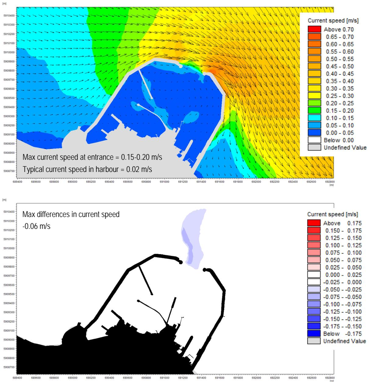
Figure 41. Baseline Tidal Current Speed (Top) and Difference in Current Speed (Bottom) as a Result of the Scheme (Mean Spring Tide, HW+1hrs, Ebb)
