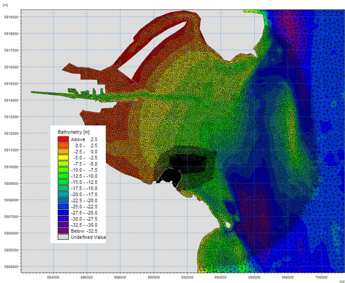
Figure 55. Detail of the Model Mesh Within Dublin Bay
