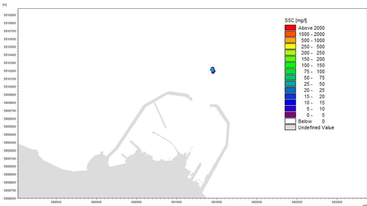
Figure 27. Increase in SSC Resulting from Continuous Dredging of Sandy Sediment outside Dun Laoghaire Harbour (Spring Tide, High Water Slack)
