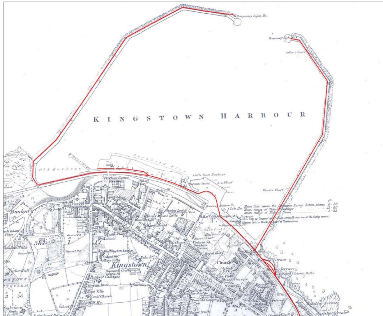
Fig. 2.35 (below) 1843: This shows the full extent of the Metals. Note the altered route of the truckway across the railway causeway, through the Old Harbour, built to carry the extension of the Dublin-Kingstown railway from Salthill to the present Dun Laoghaire Station.
