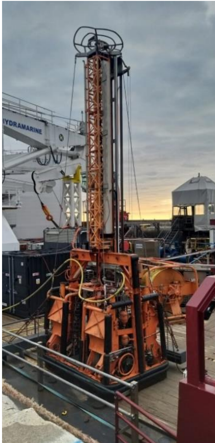
Figure 2-3: Combined Seabed rig for CPT and Vibrocore, GeoCeptor.
