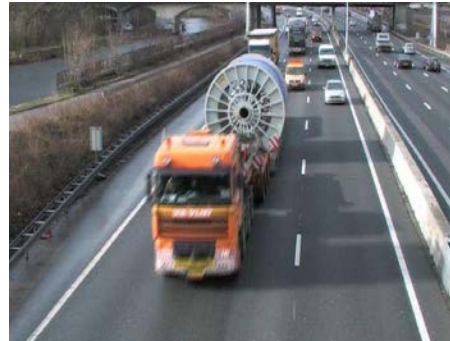
Figure 2: 400kV XLPE drums transported by truck
