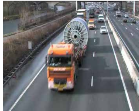
Figure 2: 400kV XLPE drums transported by truck
