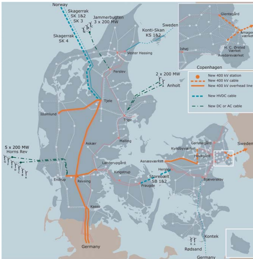
Figure 5 Expansion principle D – new 400 kV overhead lines in areas where overhead lines have already been erected, but on towers in new design.
