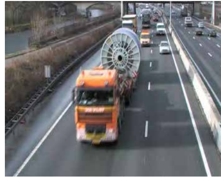
Figure 2: 400kV XLPE drums transported by truck
