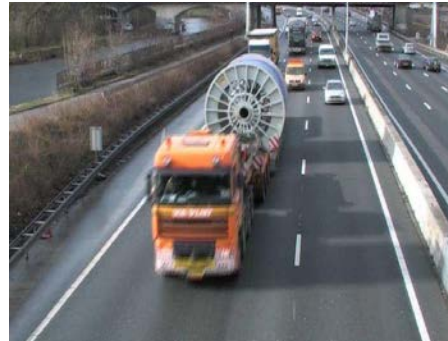
Figure 2: 400kV XLPE drums transported by truck
