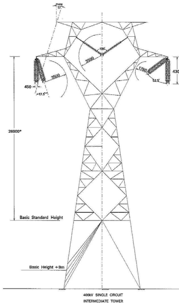
Figure 3.1 Drawing of a typical suspension tower
