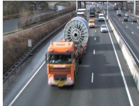
Figure 2: 400kV XLPE drums transported by truck
