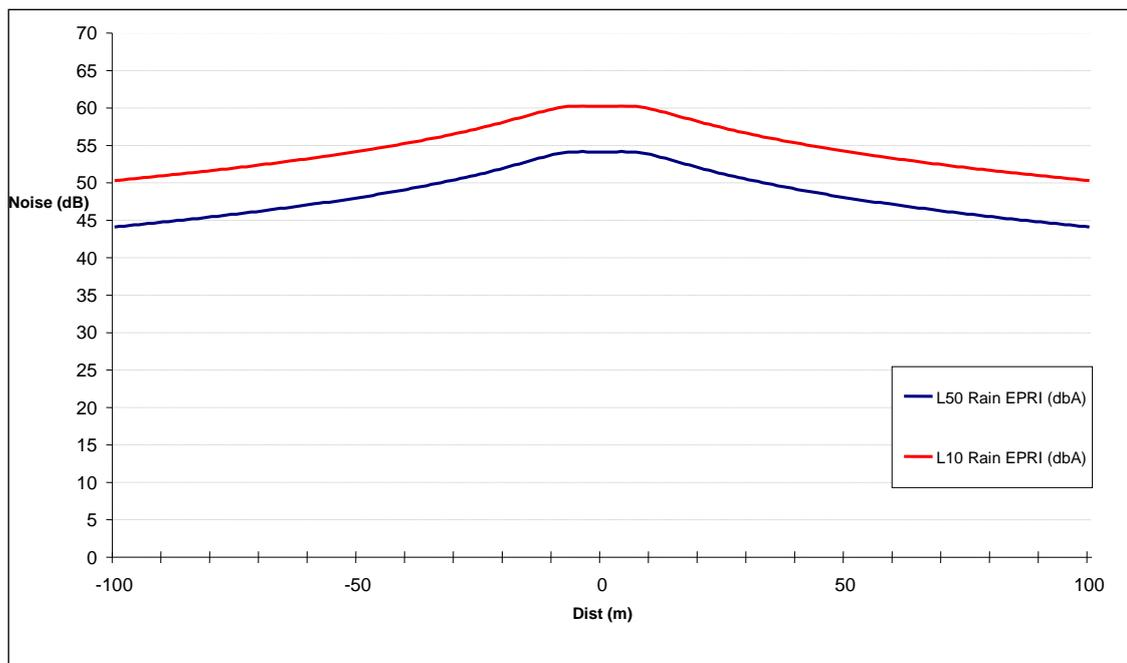
**Figure 9.2: 400 kV Double Circuit Line Noise Levels in Wet Conditions**
