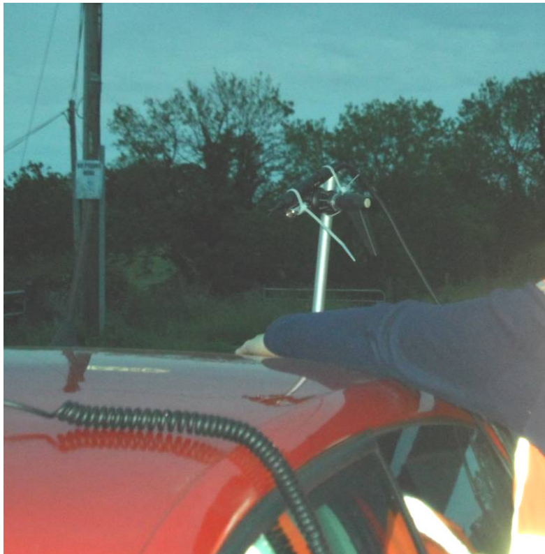
Photograph 2 – shows a more distant view of the same set up as in the close up in photo 1. Note that the external microphone is attached to the Petterson D500x full-spectrum bat detector inside the vehicle allowing the recording to be continually monitored by the passenger during the transect survey. The coiled cable in the foreground is for the flashing beacon to identify a slow moving vehicle (15mph) during survey.
