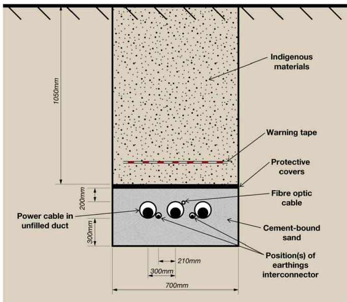
Typical Underground HVAC Arrangement
