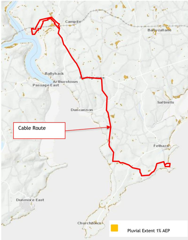
Figure 12: Cable Route vs PFRA Pluvial Extent Map ([www.myplan.ie](http://www.myplan.ie)) (not to scale)
