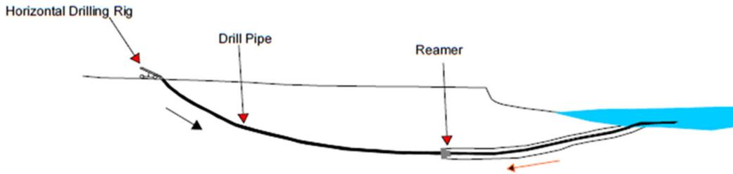
Next, a reaming tool is pulled back through the pilot hole to enlarge the hole. More than one pass may be required to make the hole larger than the diameter of the pipe
