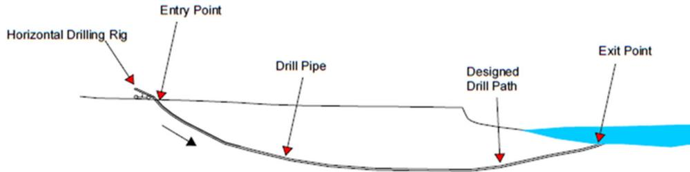
A small diameter pilot hole is drilled from the entry point, under the sea bed, to the exit point.
