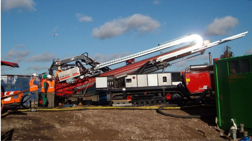
**Figure 4.7: Photo of Typical maxi-rig HDD Drill Rig**
