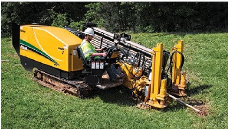
**Figure 4.10: HDD Mini-Rig**
