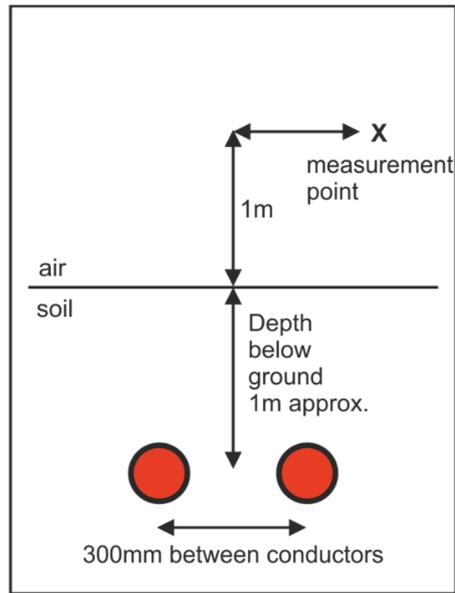
Figure 1: Cable Arrangement
