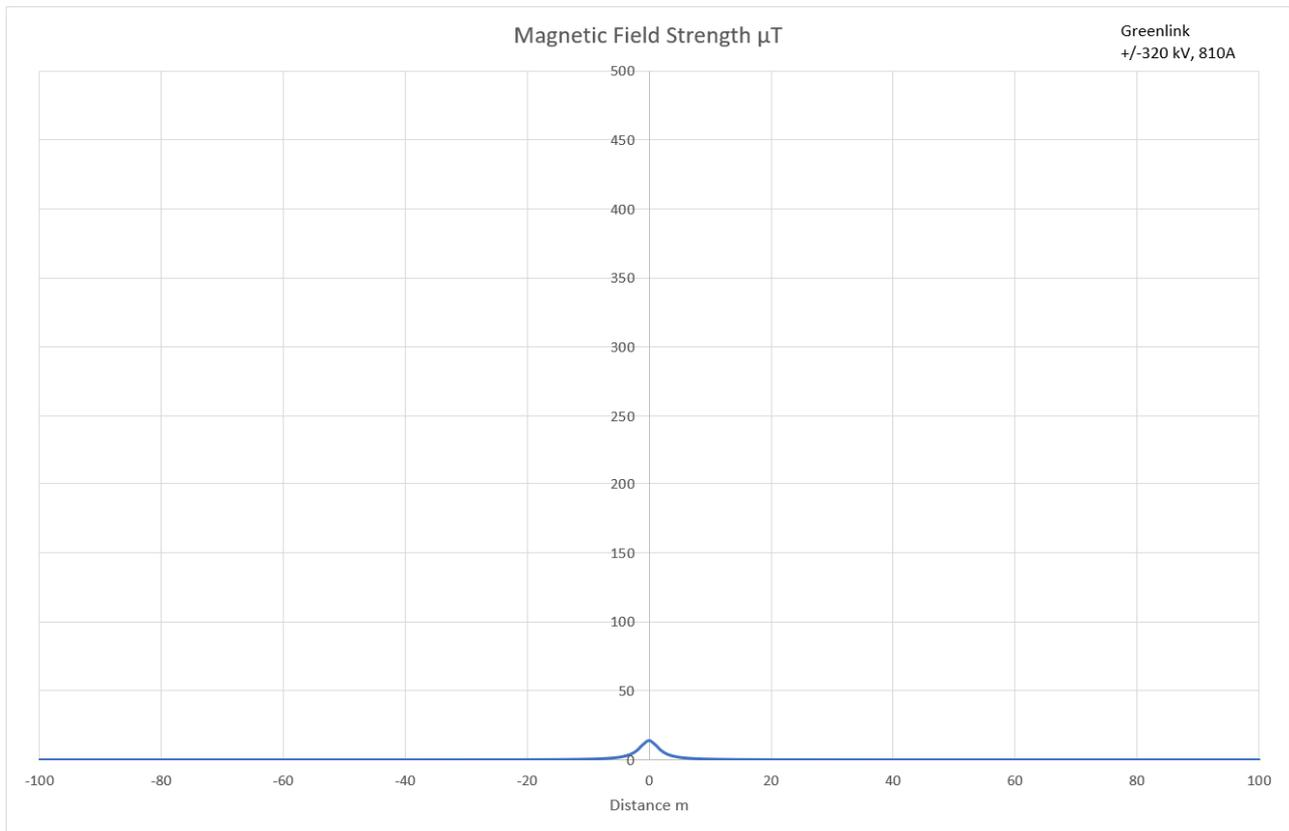
Figure 3: Magnetic Field Strength at 810 amps
