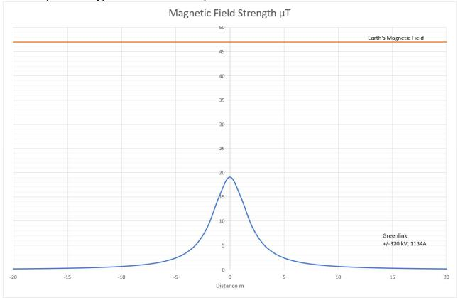
Figure 2: Magnetic Field Strength on 100% Load (1134 amps)
