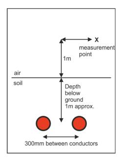
Figure 1: Cable Arrangement
