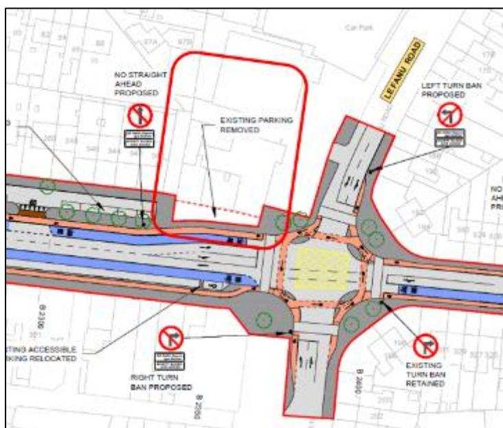
**Figure 3-34: Proposed new Layout at Grange Cross**
