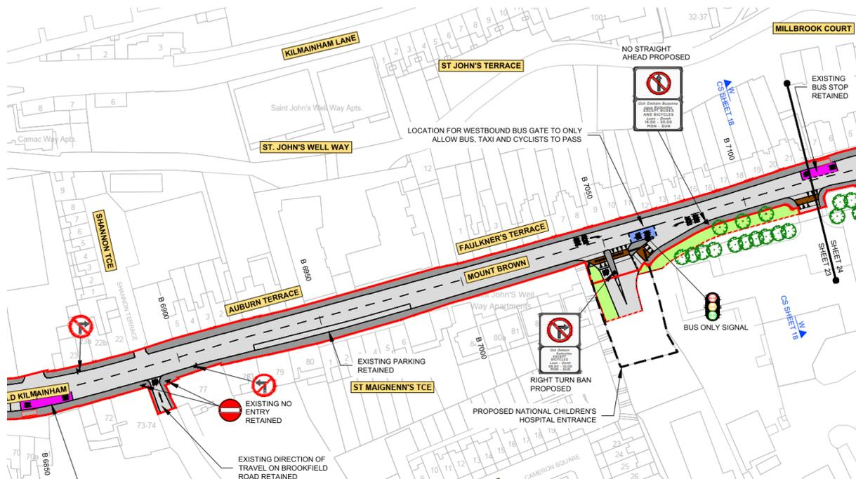
Figure 2-1: Extract 1 from General Arrangement Drawing
