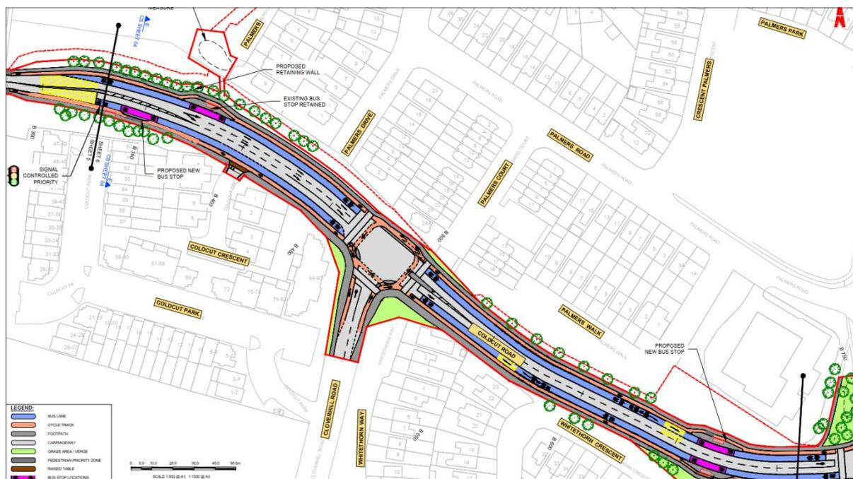
Figure 2-18: Extract 1 from General Arrangement Drawing
