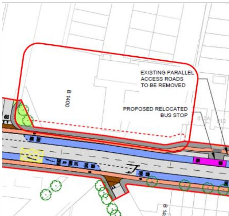
**Figure 3-49: Proposed new Layout at Applegreen Service Station**
