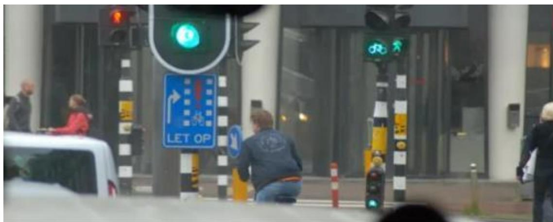
**Figure 2-42 Example from the Netherlands of traffic signals + give way signage controlling turning traffic and cyclists (Source: Dutch Design Guide Ontwerprijzer Fietsverkeer)**
