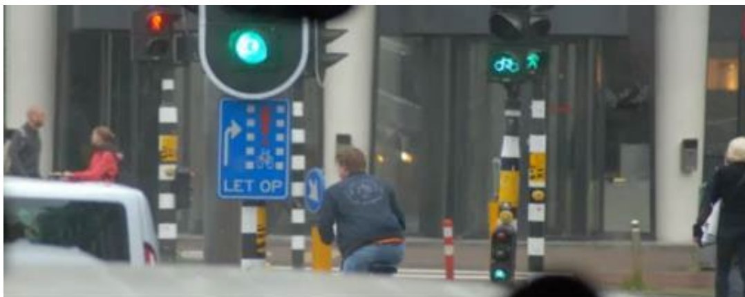
Figure 2-9-2: Example from the Netherlands of traffic signals + give way signage controlling turning traffic and cyclists (Source: Dutch Design Guide Ontwerprijzer Fietsverkeer)
