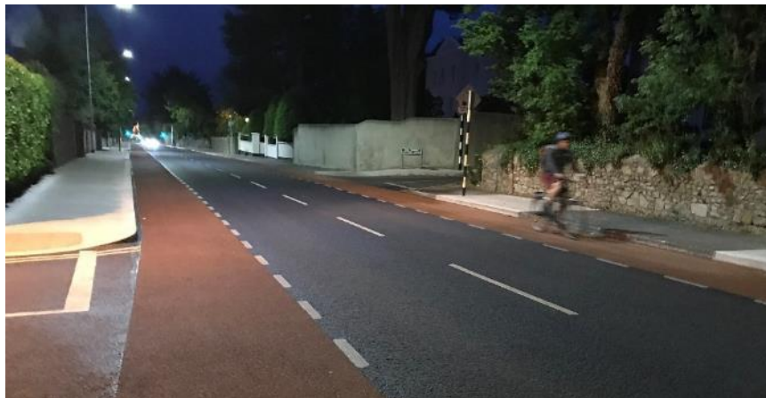
Figure 2-4-4: Example of Cycle Lanes with Red Epoxy Surfacing
