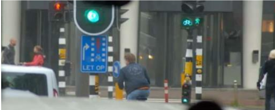
Figure 2.4.2 Example from the Netherlands of traffic signals + give way signage controlling turning traffic and cyclists (Source: Dutch Design Guide Ontwerpwijzer Fietsverkeer)
