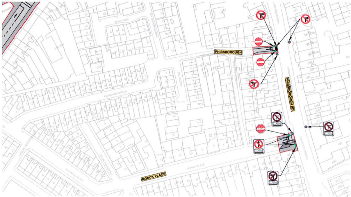
Extract of Bus Connects Plan to restrict traffic flow at Phibsborough Road, Monck Place & Avondale Avenue ('Phibsborough')
