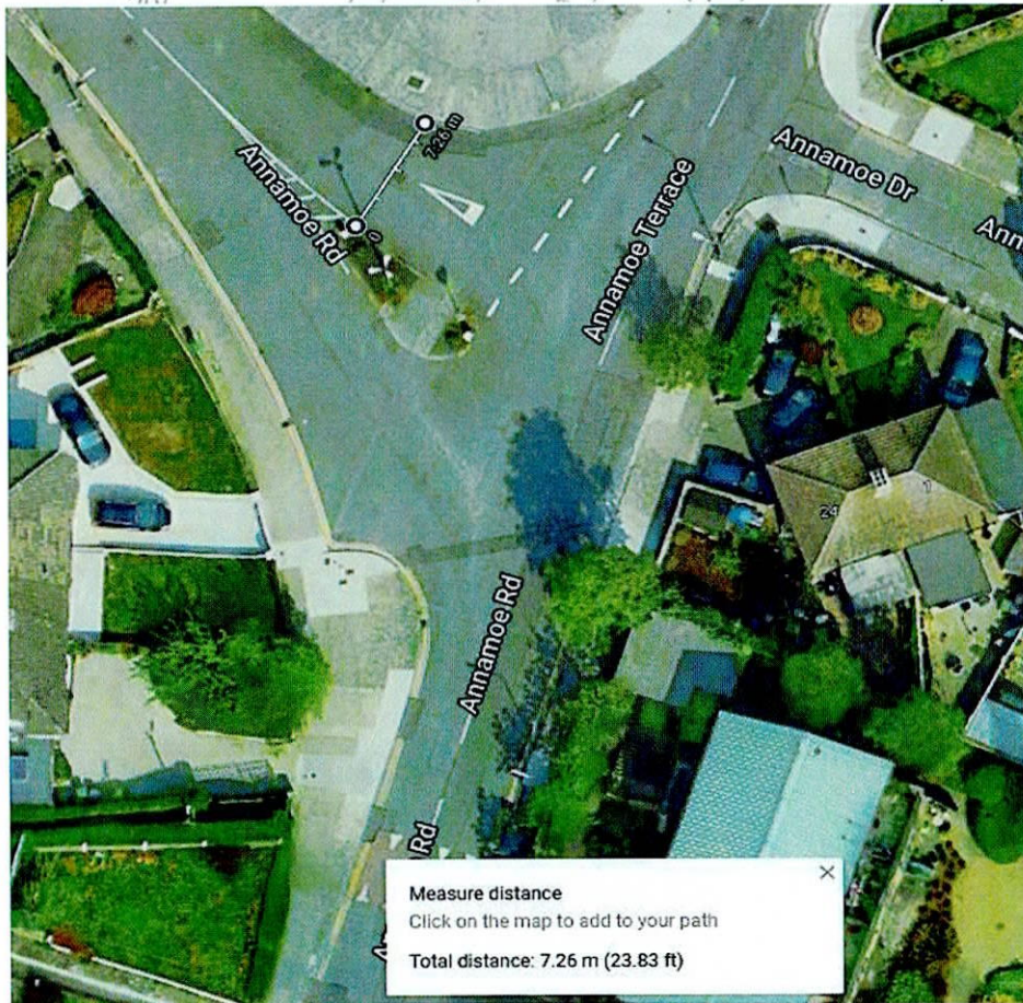
Figure 1 Above: Schematic showing Annamoe Rd & Annamoe Terrace Junction. Below: Measurement from Google Maps showing 7.26m wide for a single carriageway on Annamoe Rd
