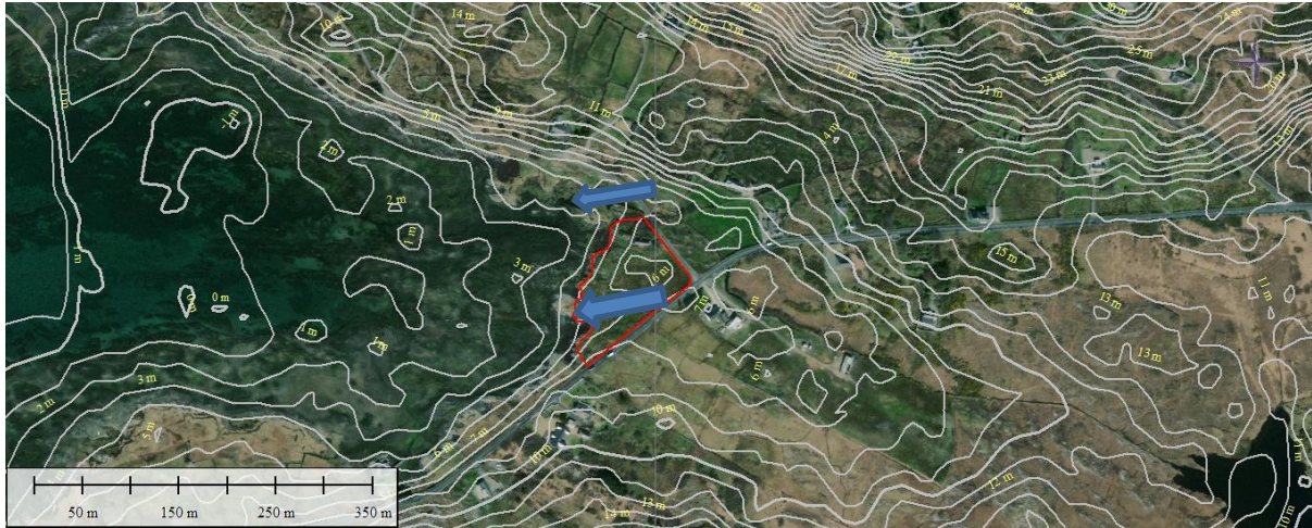
Figure 16: Natural flow paths shown on a contour map
