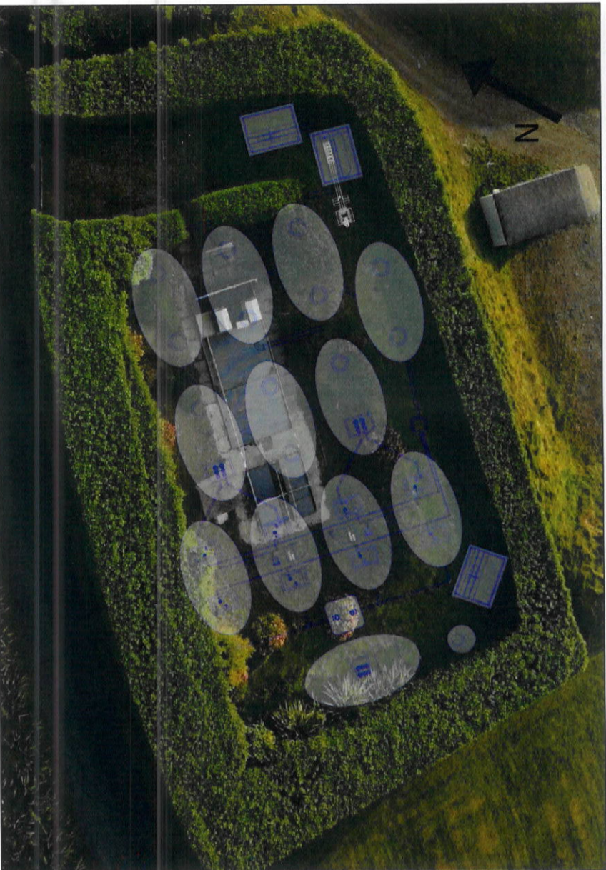
Figure 4.1: Proposed WwTP Site Layout Plan superimposed over existing WwTP. (Source: JB Barry & Partners.)
