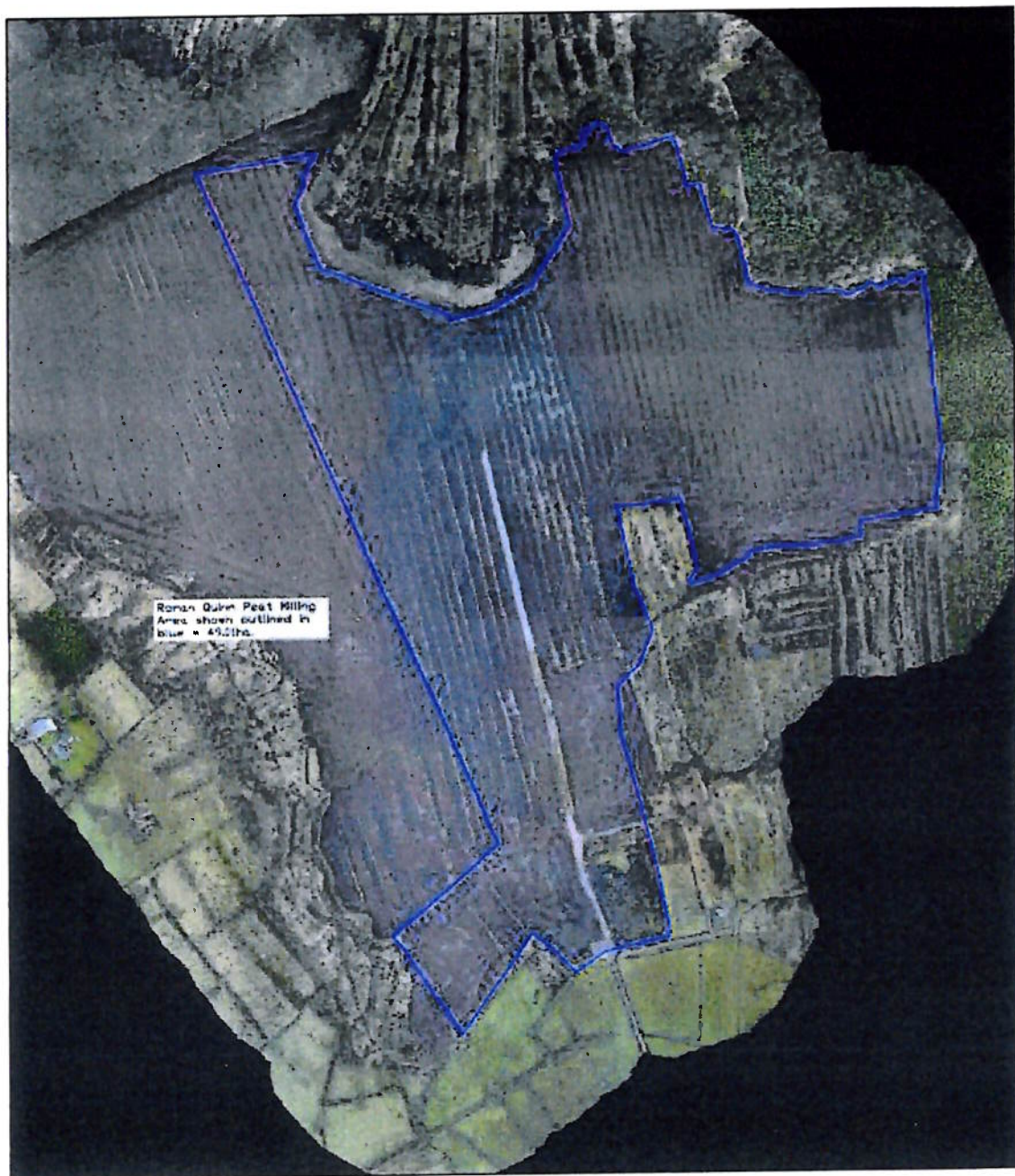
Figure 5: Ronan Quinn's property boundary, Derrymore Bog, Co. Longford. Image: Brandon O'Brien Consulting Engineers. The blue-grey strips within the property reflect those areas where the peat substrate (glacial till) has been encountered, after which milling has ceased.
